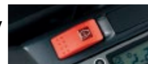
Emergency stop switch
