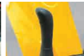
One-touch wiper switch (right lever)
